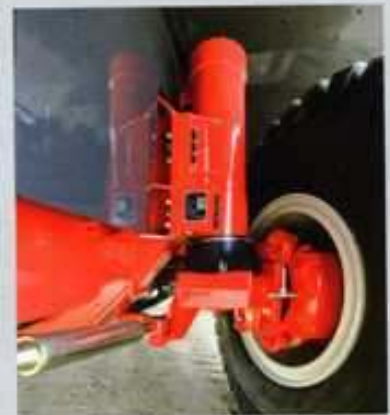
RD 50 Cilindro sosp. anteriore RD 50 Front susp. cylinder
