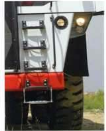
▲ RD 50 accesso in cabina frontale RD 50 frontal access into the cabin
